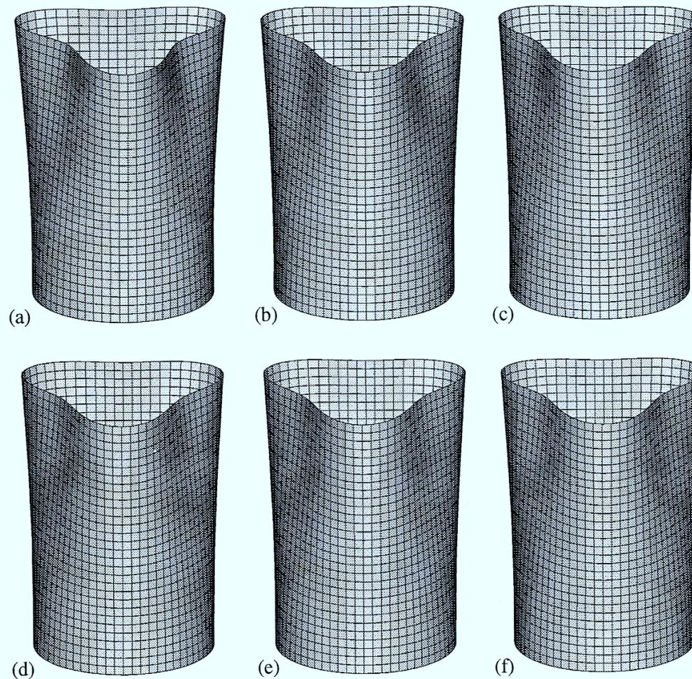
Fig. 4. Predicted mode shapes with  $m = 1$  and  $n = 3$ : (a) empty shell,  $d/L = 0$ ; (b)  $d/L = 0.2$ ; (c)  $d/L = 0.4$ ; (d)  $d/L = 0.6$ ; (e)  $d/L = 0.8$ ; (f)  $d/L = 1$ .
