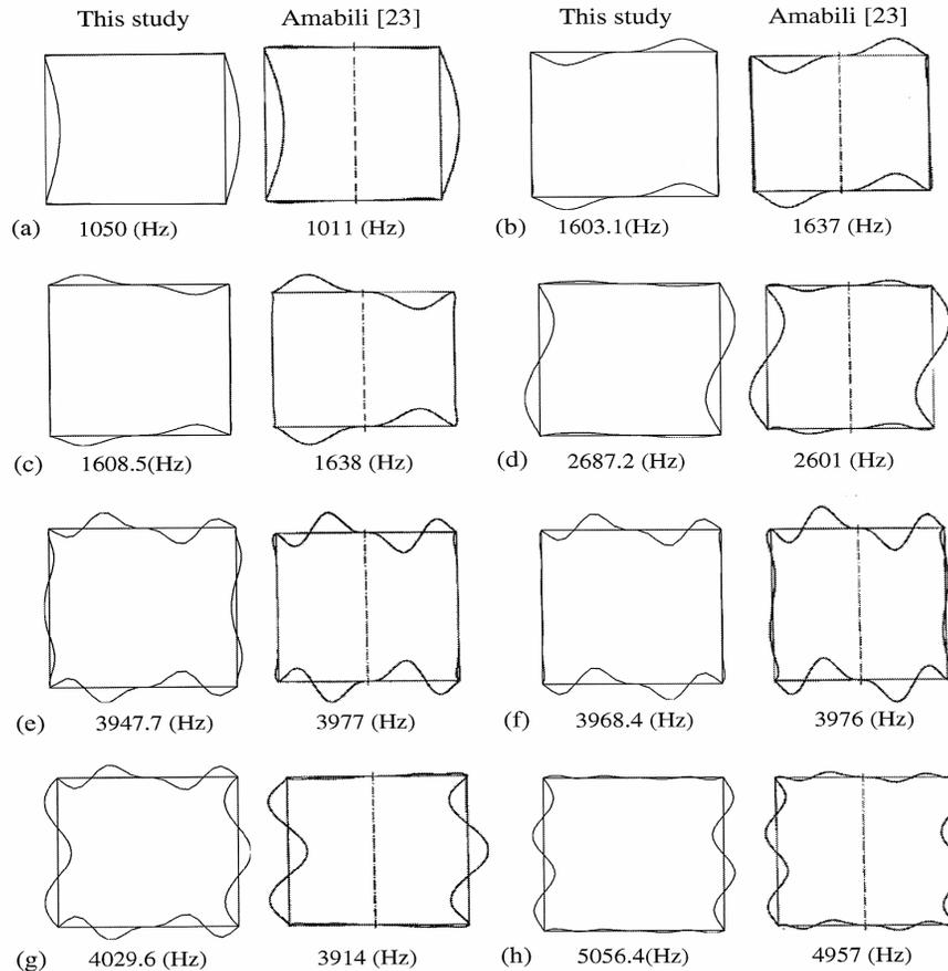
Fig. 7. Comparisons of predicted wet mode shapes of completely filled hermetic can for  $n$  (or  $i$ ) = 3: (a) first symmetric shell-dominant mode; (b) first anti-symmetric plate-dominant mode; (c) first symmetric plate-dominant mode; (d) first anti-symmetric shell-dominant mode; (e) second symmetric plate-dominant mode; (f) second anti-symmetric plate-dominant mode; (g) second symmetric shell-dominant mode; (h) second anti-symmetric shell-dominant mode.
