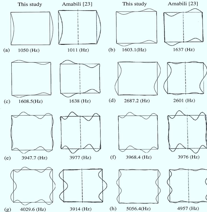
Fig. 7. Comparisons of predicted wet mode shapes of completely filled hermetic can for  $n$  (or  $i$ ) = 3: (a) first symmetric shell-dominant mode; (b) first anti-symmetric plate-dominant mode; (c) first symmetric plate-dominant mode; (d) first anti-symmetric shell-dominant mode; (e) second symmetric plate-dominant mode; (f) second anti-symmetric plate-dominant mode; (g) second symmetric shell-dominant mode; (h) second anti-symmetric shell-dominant mode.
